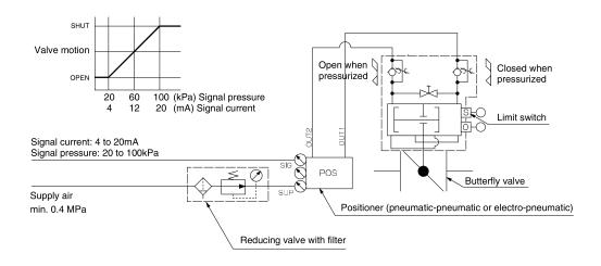
→The butterfly valve opens fully when the input signal goes off under a state of assured air supply.
