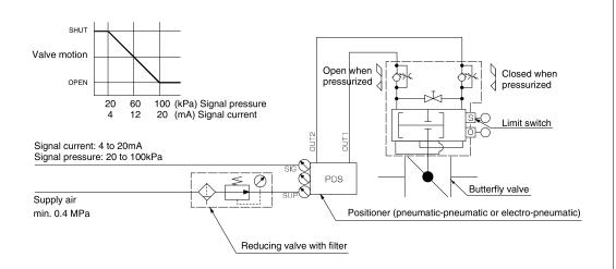
→The butterfly valve closes fully when input signal goes off under a state of assured air supply.
